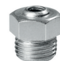
Pressure relief For releasing excessive pressure in gearboxes or bearing housings are usually made of steel, zinc-plated and passivated, with tapered thread. Available in many different types.
